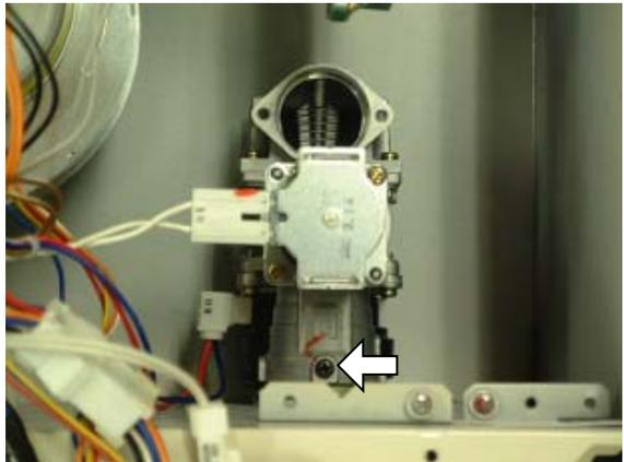
(2) Pull up the gas electromagnetic valve to the upper section and remove it.
