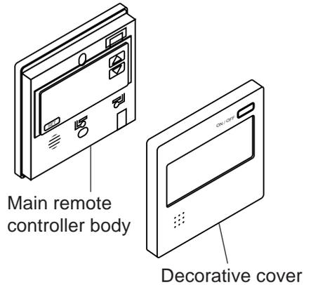
(2) Position the holes (diameter: 6 mm X depth: 25 - 30 mm) to secure the remote controller for the kitchen, and knock in all the wall anchors. Next, secure it using oval-headed wood screws.
