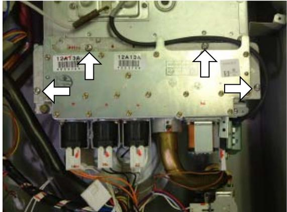
(3) Pull up and remove the manifold.
