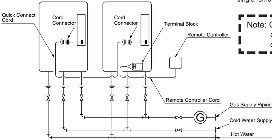
\* When connecting 2 devices, use only a single remote controller.
