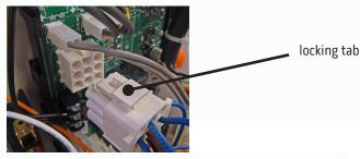
ANDREWS WATER HEATERS 5. Plug the new loom from this kit, into the honeywell control PCB and plug the original wiring connector into the new loom (see photos below)
