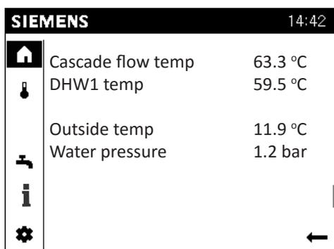
*The most important present parameters will be displayed (depending on how the system is configured).*
