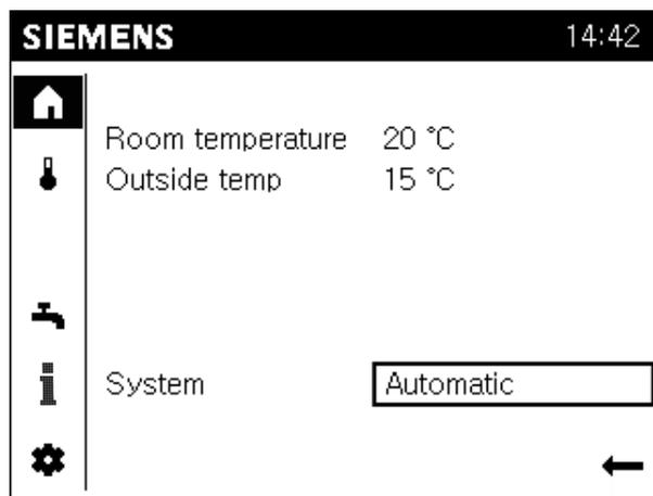
*The start page for the QAA74 room unit displays the most important information on the room and system operation mode.*
