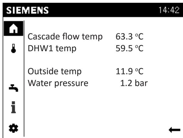
*The start page for the appliance GUI unit displays the most important information on the energy producer and system operation mode.*
