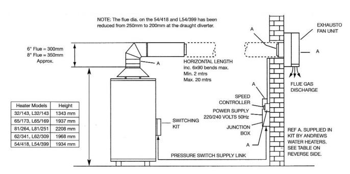
The Exhausto Flue Fan when used on Hi-Flo Water Heaters with the Remote Time Control Switching Kit will give the following control facility.
